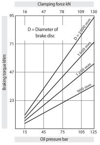
The braking torques shown in the diagram are based on a theoretical friction coefficient of 0,4.
