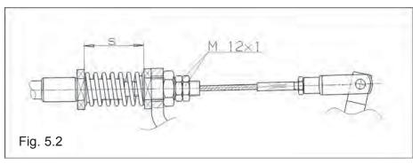
The compensation spring is pre-tensed to dimension s = 50 mm by the 2 nuts (M12x1). (At this setting, the handbrake lever must not to be in self-arresting position over the zero point.)
