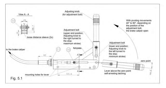
The pull cable is connected to the handbrake lever by the manufacturer. The pull cable can be detached if necessary using the following procedure:
